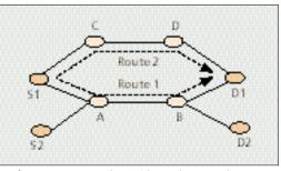
Figure 1. A simple problem of route selection. Selecting the route (S<sub>1</sub>, C, D, D<sub>1</sub>) leaves link (A, B) free for future QVPNs between S<sub>2</sub> and D<sub>2</sub>.
