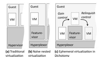
Figure 1: Splitting the role of the hypervisor with ephemeral virtualization
