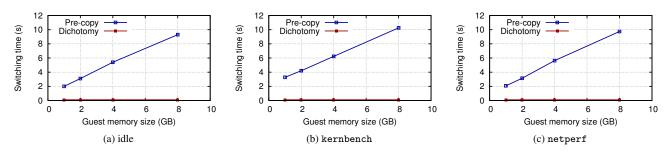
Figure 13: Switching times of guest VMs with varying memory sizes between hyperplexor to featurevisor.
