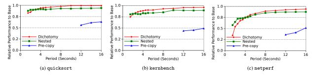
Figure 11: Workload runtimes when switching between hyperplexor and a featurevisor running the netmon task.
